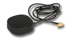
The RF-3070-AT242 is a portable, active L1/L2 GPS antenna with an integrated pendant coaxial cable and magnetic mount. The 3-foot long RG-174 coaxial cable terminates in a right angle SMB connector for direct connection to the AN/PRC-117G(V)1(C) and RF-7800M-MP Falcon III® manpack transceivers. The magnetic mount has a retaining force of approximately 18 lbs.
